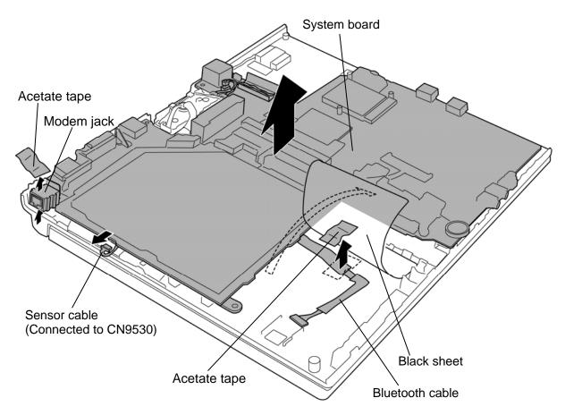
Figure 4-37 Removing the system board (2)
